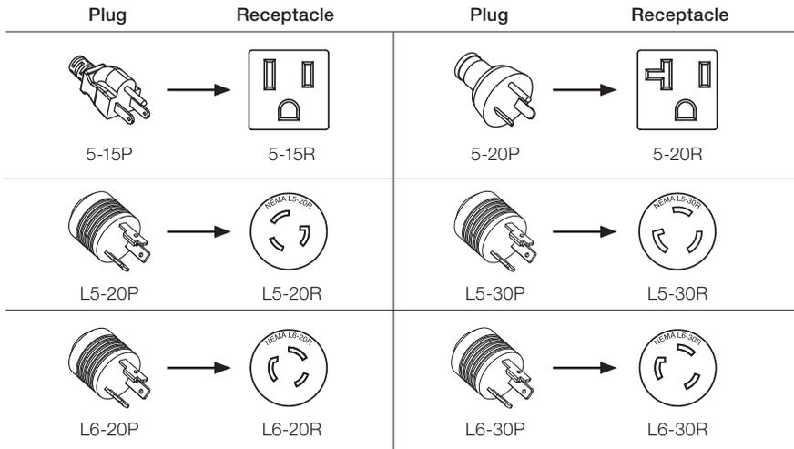
**Note:** Locking plugs and receptacles are not interchangeable. For example an L6-20P plug will not lock into an L6-30R receptacle.
