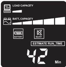
The LCD display panel provides critical load and battery information. (2U/5U LCD Screen Shown)
