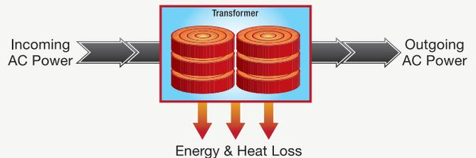
The transformer in a conventional line-interactive UPS loses significant energy as heat is generated during normal utility power output.
