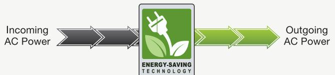
GreenPower UPS Technology bypasses the transformer when utility power is normal, reducing energy consumption and heat loss.
