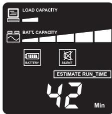
The LCD display panel provides critical load and battery information. (2U LCD Screen Shown)
