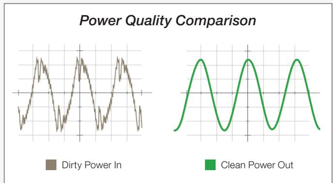
Computers incorporating Active PFC power supplies in their design architecture require optimal power quality to function properly.
