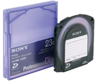
The Professional Disc™ is a single-sided, optical disc that uses state-of-the-art blue violet laser technology. Despite its small size, the disc provides an amazing storage capacity of 23.3 GB – a feat made possible using a 405 nm blue-violet laser and an object lens with a 0.85 numerical aperture (NA) and specially developed recording layer.
