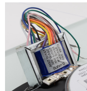
70/25V transformer with colored leads
