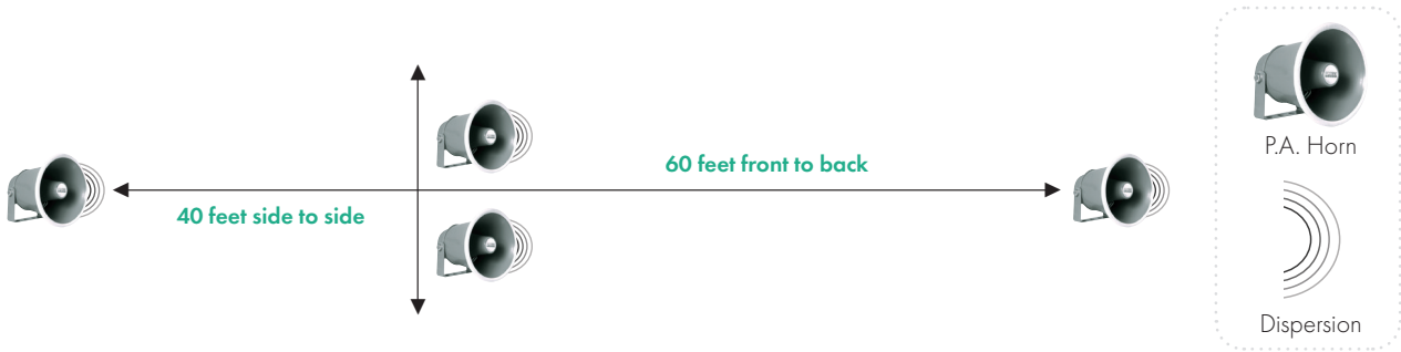
Diagram 5: Proper Placement of P.A. Horns in "Diamond Pattern"
