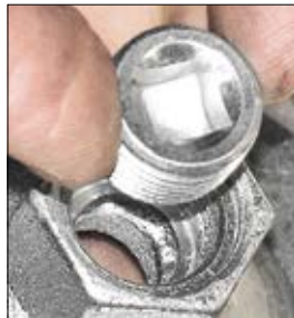
NO-SLIP SQUARE-HEAD DRIVER TO TIGHTEN
