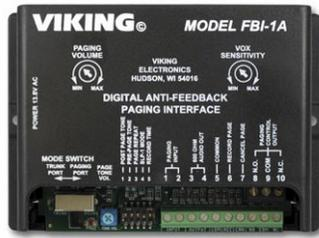
**HOW IT WORKS:** The “live” page is digitally recorded. When complete, the paging amplifier is activated and the page is replayed once or twice.
