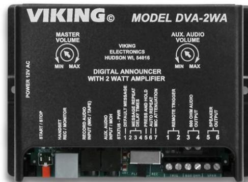
The **DVA-2WA** is a digital announcer/recorder with a built in 2 Watt amplifier. Designed to provide music and promotion on hold, the **DVA-2WA** can playback in a continuous loop or alternate between promotions and an auxiliary music source at 2 second to 30 minute intervals. Any number of multiple messages may be recorded.
