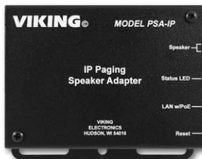
The **PSA-IP** has a high efficiency 6 Watt class D amplifier capable of driving up to six 8 Ohm analog paging speakers.
