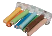
Wires protrude from the front of the connector before being trimmed flush.
